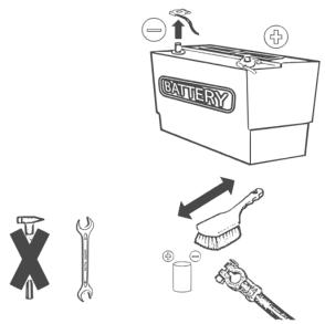
3.2 Remove the electrical connecting cables from the currently installed alternator. Carefully mark the connecting cables according to the associated output terminals on the alternator.
