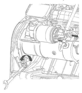
3.5 Make sure that the new starter motor matches the starter motor you just removed. Compare the number of teeth, the flange design, the electrical connections, the rated voltage, the direction of rotation, etc.
