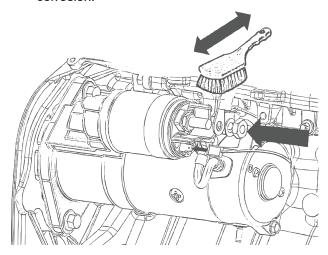
3.7 Install the starter motor on the engine and properly tighten the fixing bolts. Follow the vehicle manufacturer's instructions.
